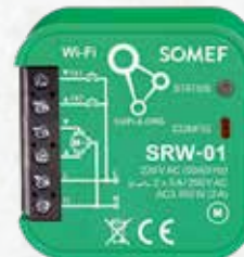
SRW-01 Shutters control
