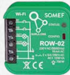
ROW-02 Lighting control for tow circuits
